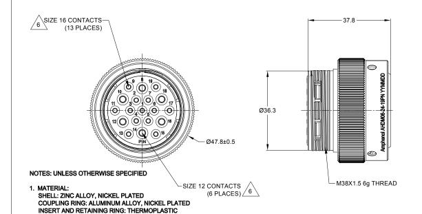
2. MODIFICATIONS: THREADED HOUSING; NORMAL DIA. WIRE SEAL
