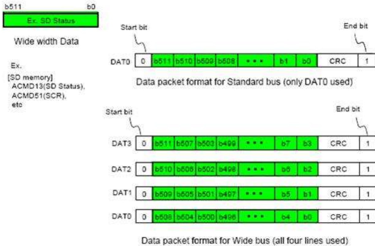
Figure 6-1-7: Data packet format - Wide width data
