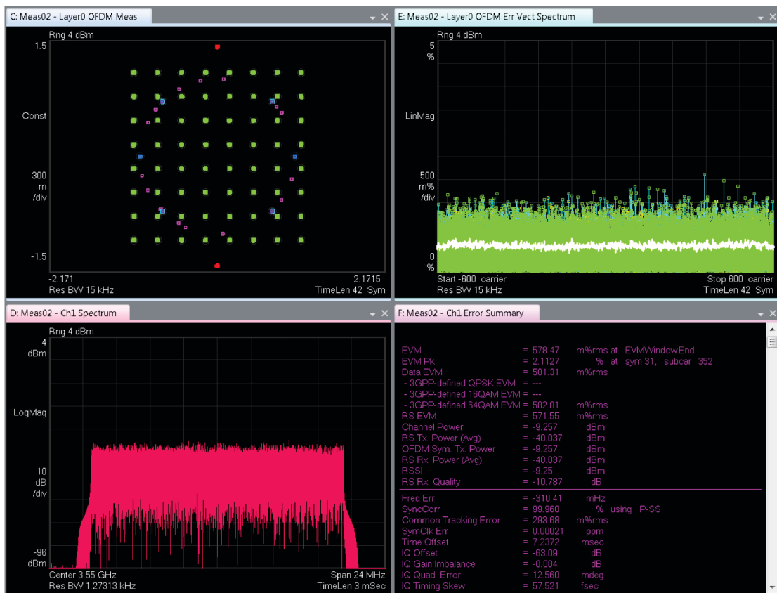
Figure 260. Observed EVM Before Applying CFR
