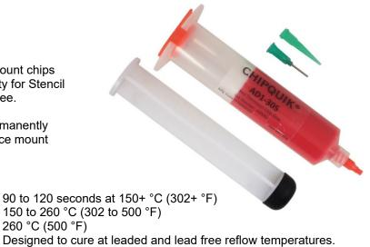
150 to 260 °C (302 to 500 °F) 260 °C (500 °F) Designed to cure at leaded and lead free reflow temperatures. -40 to 125 °C (-40 to 257 °F) (After Curing, After Reflow) >15MPa (Steel-Steel, 25 °C (77 °F)) 1.25g/cc 450,000 mPa-s 80°C 60x10^-6/K (60 ppm/°C) 120x10^-6/K (120 ppm/°C) 0.14 W/(m·K) 25 KV/mm (at 25°C) 3.2 (at 25°C, 1MHz) <0.02 (at 25°C, 1MHz) <10% 30cc/30g Syringe Refrigerated >3 months, Unrefrigerated >3 months
