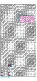
₩ Welding paint Bottom Layer ■ Bare copper area
