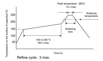
Soldering temperature and soldering time
