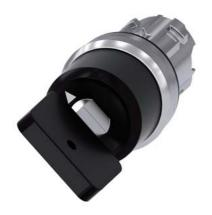
key-operated switch Siemens, 22 mm, round, metal, shiny, lock no. VL5, with 2 keys, 2 switch positions O-I, latching, actuating angle 90°, 10:30h/13:30h, key removal O, with laser labeling, upper case and lower case, always upper case at beginning of line
