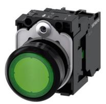
Illuminated pushbutton, 22 mm, round, plastic, green, pushbutton, flat, momentary contact type, with holder, 1NO, LED module with integrated LED 24 V AC/DC, screw terminal, with laser labeling, upper case and lower case, always upper case at beginning of line
