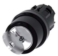
RONIS key-operated switch, 22 mm, round, plastic, lock number SB30, with 2 keys, 2 switch positions O-I, latching, actuating angle 90°, 10:30h/13:30h, key removal O+I, possible special locks: SB31, 421, 455, with laser labeling, upper case
