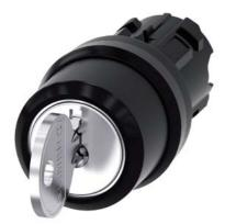
RONIS key-operated switch, 22 mm, round, plastic, lock number SB30, with 2 keys, 3 switch positions I-O<II, left latching, right momentary contact type, actuating angle  $2x45^{\circ}$ , 10:30h/12h/13:30h, key removal O+I, possible special locks: SB31, 421, 455, with laser labeling, upper case
