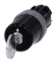
Key-operated switch BKS, 22 mm, round, plastic with metal front ring, lock number S1, with 2 keys, 3 switch positions I-O<II, left latching, right momentary contact type, actuating angle 2x45°, 10:30h/12h/13:30h, key removal I, with laser labeling, Customer-specific selection with SIRIUS ACT configurator (CIN)
