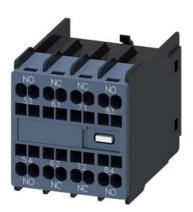
auxiliary switch front-side, 2 NO + 2 NC current path 1 NO, 1 NC, 1 NC, 1 NO for contactor relays size S00 spring-loaded terminal 53/54, 61/62, 71/72, 83/84 physically coded; only combinable with contactor relays 3RH2140\* and 3RH2440\* (according to EN 50011)
