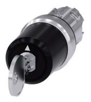
Key-operated switch BKS, 22 mm, round, metal, shiny, lock number S1, with 2 keys, 3 switch positions I-O<II, left latching, right momentary contact type, actuating angle 2x45°, 10:30h/12h/13:30h, key removal O, with laser labeling, upper case and lower case, always upper case at the beginning of the word
