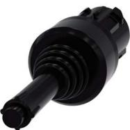
Coordinate switch, 22 mm, round, plastic, black, 4 switch positions, latching, with mechanical interlocking, with laser labeling, inscription or symbol, Customer-specific selection with SIRIUS ACT configurator (CIN)
