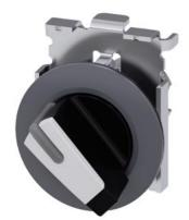
Selector switch, illuminable, 30 mm, round, Metal, matte, white, selector switch, short, front ring for flush installation, 2 switch positions O<I, momentary contact type, Actuating angle 45°, 10:30h/12h, Z=50-unit packaging
