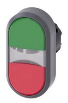
Illuminated twin pushbutton, 22 mm, round, plastic with metal front ring, green, red, pushbuttons, flat, with laser labeling, upper case and lower case, always upper case at the beginning of the word
