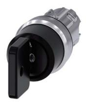
Key-operated switch O.M.R, 22 mm, round, metal, shiny, lock number 73034, black, with 2 keys, 3 switch positions I-O-II, latching, actuating angle 2x45°, 10:30h/12h/13:30h, key removal O, with laser labeling, upper case and lower case, always upper case at the beginning of the word
