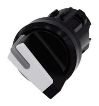
Selector switch, illuminable, 22 mm, round, plastic, white, selector switch, short, 2 switch positions O-I, latching, actuating angle 90°, 10:30h/13:30h, with laser labeling, inscription or symbol Customer-specific selection with SIRIUS ACT configurator (CIN)
