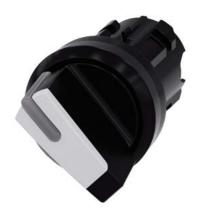
Selector switch, illuminable, 22 mm, round, plastic, white, selector switch, short, 2 switch positions O<I, momentary contact type, Actuating angle 45°, 10:30h/12h, with laser labeling, upper case
