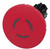
EMERGENCY STOP mushroom pushbutton, illuminable, 22 mm, round, plastic, red, 60 mm, positive latching, acc. to EN ISO 13850, rotate-tounlatch, with laser labeling, upper case and lower case, always upper case at beginning of line
