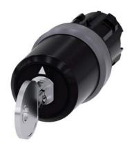
key-operated switch Siemens, 22 mm, round, plastic with metal front ring, lock number SSG10, with 2 keys, 3 switch positions I-O-II, latching, actuating angle 2x45°, 10:30h/12h/13:30h, key removal I+II, with laser labeling, lower case
