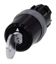
key-operated switch Siemens, 22 mm, round, plastic with metal front ring, lock number SSG10, with 2 keys, 3 switch positions I-O<II, left latching, momentary contact type on the right, actuating angle  $2x45^{\circ}$ , 10:30h/12h/13:30h, key removal O, with laser labeling, upper case and lower case, always upper case at beginning of line
