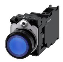
Illuminated pushbutton, 22 mm, round, plastic, blue, pushbutton, flat, momentary contact type, with holder, 1 NO+1 NC, LED module with integrated LED 24 V AC/DC, spring-type terminal, with laser labeling, inscription or symbol Customer-specific selection with SIRIUS ACT configurator (CIN)
