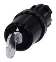
Key-operated switch BKS, 22 mm, round, plastic, lock number S1, with 2 keys, 3 switch positions I>O<II, momentary contact type, actuating angle 2x45°, 10:30h/12h/13:30h, key removal O, with laser labeling, upper case and lower case, always upper case at beginning of line
