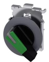
Selector switch, illuminable, 30 mm, round, Metal, matte, green, selector switch, long, front ring for flush installation, 2 switch positions O<I, momentary contact type, Actuating angle 45°, 10:30h/12h, with laser labeling, upper case
