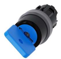
Key-operated switch O.M.R, 22 mm, round, plastic with metal front ring, lock number 73038, blue, with 2 keys, 2 switch positions O<I, momentary contact type, Actuating angle 45°, 10:30h/12h, key removal O, with laser labeling, inscription or symbol Customer-specific selection with SIRIUS ACT configurator (CIN)
