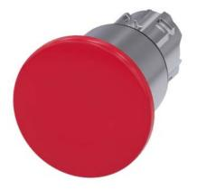
Mushroom pushbutton, 22 mm, round, metal, shiny, red, 40 mm, 3 switch positions, latches after pushing in, unlatches by pull-to-unlatch mechanism to center position, after pulling out the button Retraction to center position, with laser labeling, lower case
