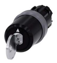
key-operated switch Siemens, 22 mm, round, plastic with metal front ring, lock number SSG10, with 2 keys, 3 switch positions I-O-II, latching, actuating angle 2x45°, 10:30h/12h/13:30h, key removal II, with laser labeling, inscription or symbol customer-specific selection with SIRIUS ACT configurator (CIN)
