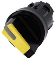
Selector switch, illuminable, 22 mm, round, plastic, yellow, selector switch, short, 2 switch positions O-I, latching, actuating angle  $90^{\circ}$ , 10:30h/13:30h, with laser labeling, lower case
