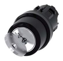
RONIS key-operated switch, 22 mm, round, plastic, lock number SB30, with 2 keys, 2 switch positions O-I, latching, actuating angle 90°, 10:30h/13:30h, key removal I, possible special locks: SB31, 421, 455, with laser labeling, upper case
