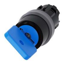
Key-operated switch O.M.R, 22 mm, round, plastic with metal front ring, lock number 73038, blue, with 2 keys, 2 switch positions O-I, latching, actuating angle 90°, 10:30h/13:30h, key removal O+I, with laser labeling, lower case
