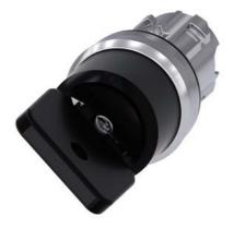
Key-operated switch O.M.R, 22 mm, round, metal, shiny, lock number 73034, black, with 2 keys, 2 switch positions O-I, latching, actuating angle 90°, 10:30h/13:30h, key removal I, with laser labeling, upper case and lower case, always upper case at the beginning of the word
