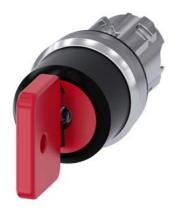
Key-operated switch O.M.R, 22 mm, round, metal, shiny, lock number 73037, red, with 2 keys, 3 switch positions I-O-II, latching, actuating angle 2x45°, 10:30h/12h/13:30h, Key removal I+O+II, with laser labeling, upper case
