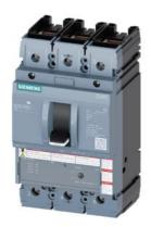
circuit breaker 3VA5 UL frame 250 3-pole, starter protection TM120M, AM, In=200A without overload protection short-circuit protection li=6...12 x In cable connection on both sides
