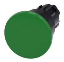
Mushroom pushbutton, 22 mm, round, plastic, green, 40mm, latching, pull-to-unlatch mechanism, with laser labeling, upper case and lower case, always upper case at the beginning of the word
