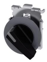
Illuminable selector switch, 30 mm, round, Metal matt, black, Selector switch long, front ring for flush installation, latching, actuating angle 90°, 10:30 /13:30, Z=50-unit packaging
