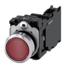
Illuminated pushbutton, 22 mm, round, metal, shiny, red, pushbutton, flat, momentary contact type, with holder, 1 NO+1 NC, LED module with integrated LED 24 V AC/DC, spring-type terminal, with laser labeling, inscription or symbol Customer-specific selection with SIRIUS ACT configurator (CIN)
