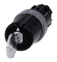
key-operated switch Siemens, 22 mm, round, plastic with metal front ring, lock number SSG10, with 2 keys, 3 switch positions I>O<II, momentary contact on the left, latching on the right, actuating angle 2x45°, 10:30h/12h/13:30h, key removal II, with laser labeling, inscription or symbol customer-specific selection with SIRIUS ACT configurator (CIN)
