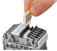
**Removing a push-in type jumper bar:**
