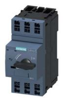
Circuit breaker size S00 for starter combination Rated current 8 A N-release 104 A Spring-type terminal Standard switching capacity
