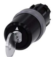
key-operated switch Siemens, 22 mm, round, plastic with metal front ring, lock number SSG10, with 2 keys, 3 switch positions I>O<II, momentary contact on the left, latching on the right, actuating angle 2x45°, 10:30h/12h/13:30h, key removal II, with laser labeling, lower case
