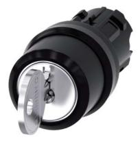
RONIS key-operated switch, 22 mm, round, plastic, lock number SB30, with 2 keys, 3 switch positions I>O<II, momentary contact type, actuating angle 2x45°, 10:30h/12h/13:30h, key removal O, possible special locks: SB31, 421, 455, with laser labeling, upper case and lower case, always upper case at beginning of line
