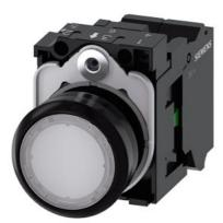
Illuminated pushbutton, 22 mm, round, plastic, white, pushbutton, flat, momentary contact type, with holder, 1NO, LED module with integrated LED 230 V AC, spring-type terminal, with laser labeling, upper case
