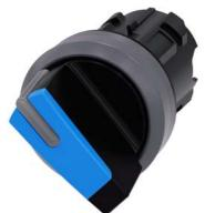
Selector switch, illuminable, 22 mm, round, plastic with metal front ring, blue, selector switch, short, 2 switch positions O-I, latching, actuating angle 90°, 10:30h/13:30h, with laser labeling, inscription or symbol Customer-specific selection with SIRIUS ACT configurator (CIN)
