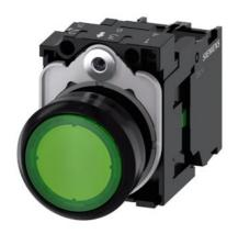
Illuminated pushbutton, 22 mm, round, plastic, green, pushbutton, flat, momentary contact type, with holder, 1NO, LED module with integrated LED 110 V AC, screw terminal, Z=20-unit packaging
