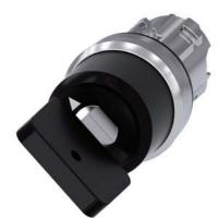
key-operated switch Siemens, 22 mm, round, metal, shiny, lock no. VL5, with 2 keys, 2 switch positions O-I, latching, actuating angle  $90^{\circ}$ , 10:30h/13:30h, key removal O, with laser labeling, upper case and lower case, always upper case at the beginning of the word
