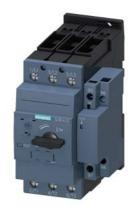
Circuit breaker size S2 for motor protection, CLASS 10 with overload relay function A-release 32...40 A N-release 585 A Standard switching capacity
