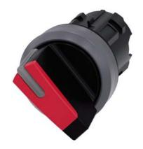
Selector switch, illuminable, 22 mm, round, plastic with metal front ring, red, selector switch, short, 2 switch positions O-I, latching, actuating angle  $90^\circ$ , 10:30h/13:30h, with laser labeling, lower case
