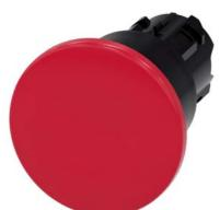
Mushroom pushbutton, 22 mm, round, plastic, red, 40mm, latching, pull-to-unlatch mechanism, with laser labeling, lower case
