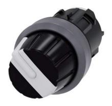
Selector switch, 22 mm, round, plastic with metal front ring, white, Rotary knob, 4 switch positions I-II-III-IV, latching, Actuating angle 4x90°, 3h/6h/9h/12h, with laser labeling, upper case and lower case, always upper case at beginning of line
